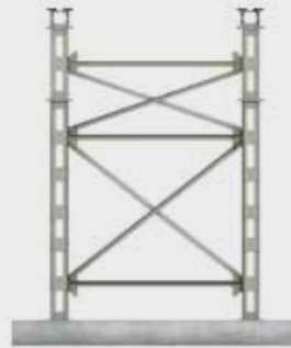
Tower Elevation Assembly
